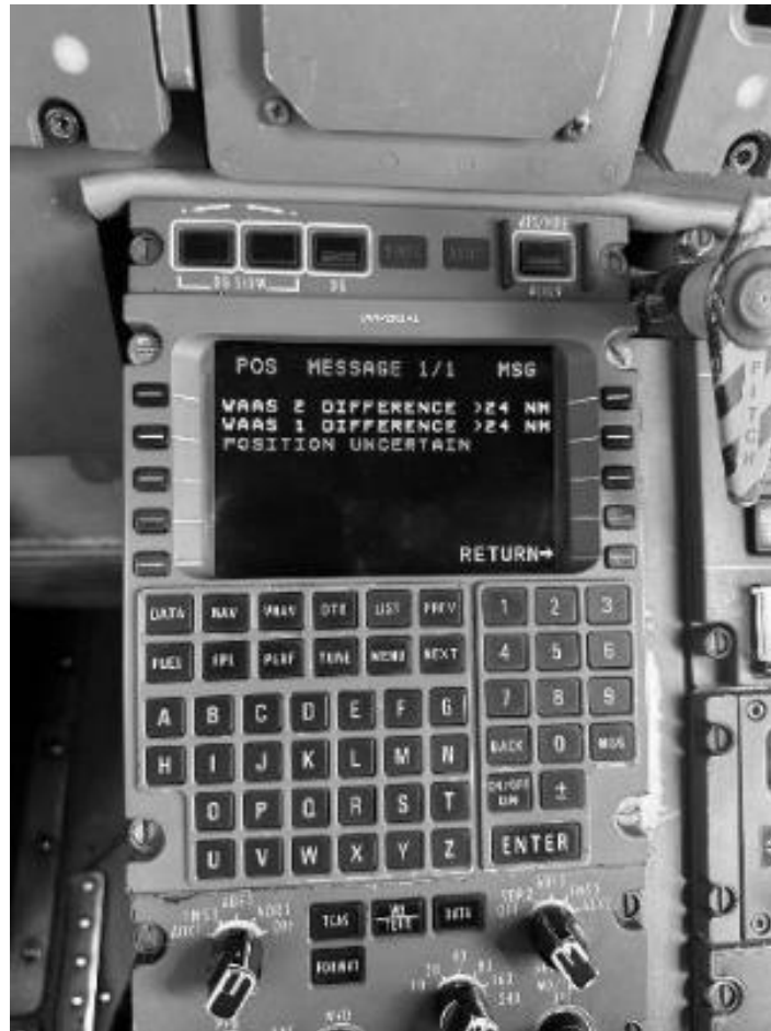
Picture of a Flight Management System Control Display Unit (FMS CDU) of a plane landing in Bujumbura, indicating “position uncertain” following jamming on 13/1/2026. Confidential source.
